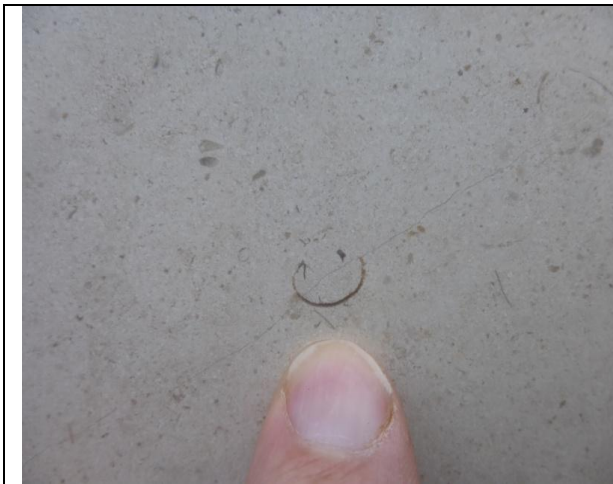
A buff coloured oolitic limestone, packed with oolites in a marl matrix with occasional shells This is thought to be Middle Jurassic Candeeiros Limestone from Porto de Mos, Portugal.
