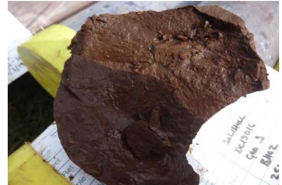
248.62 m Claystone. Grey brown to dark red brown blocky, slickenside surfaces crumbles in hand - fracture zone
